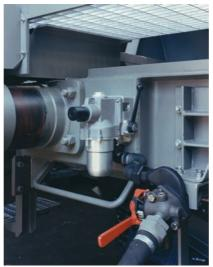
Derailing detectors are fitted to buffer beam at each end of the car and are pneumatically connected to the train's main air line via a 1"-line.
