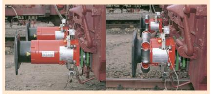
Example of a crash buffer before and after deformation. © Photo EST Railway-Systemtechnik GmbH
