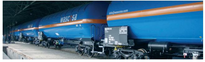
Pressurized gas tank cars are identified by the orange warning stripe around the tank and are used for various gases. A differentiation is made between the following gases:
