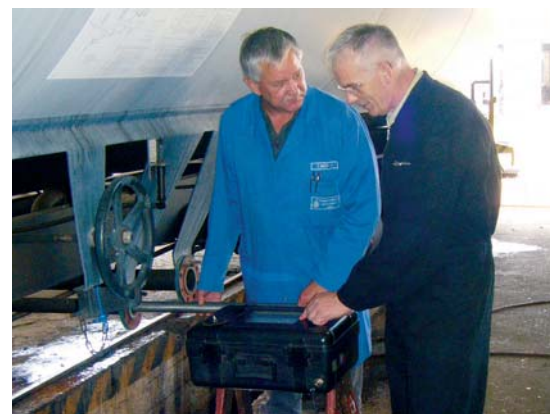
A job for specialists: endoscopic test of the drain pipes of a WASCOSA pressurized gas tank car in a specialist workshop. © Franz Kaminski Waggonbau GmbH
