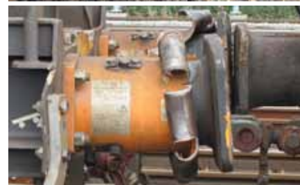
Collision in Barendrecht: picture of an intact and a deformed crash buffer.
