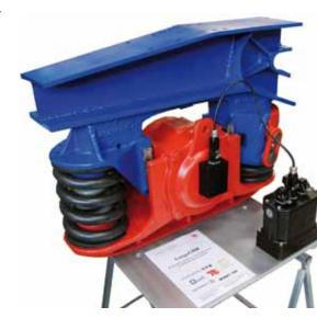
Model of data collection on the axle bearing cover and data transmission to the processing and storage box
