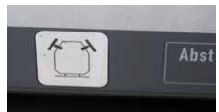
Figure 3: Pictograph on two-tier passenger car as shown Figure 2 indicating the necessary profile extension from G2 to GC
