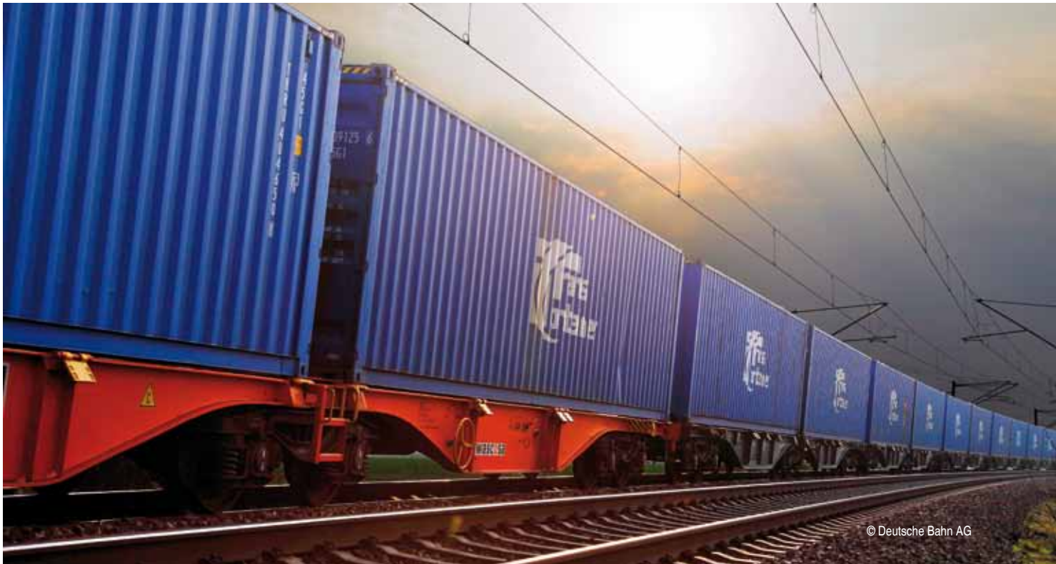
Container cars do not make the best use of the structure gauge.
