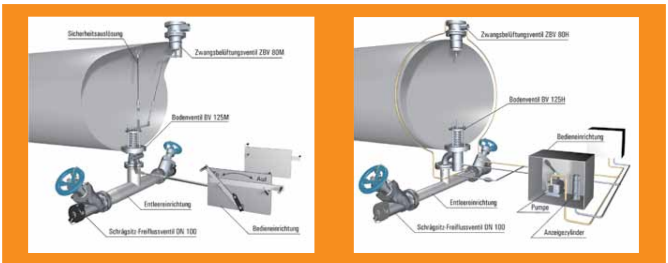
A mechanical system is shown on the left and a hydraulic one on the right.
