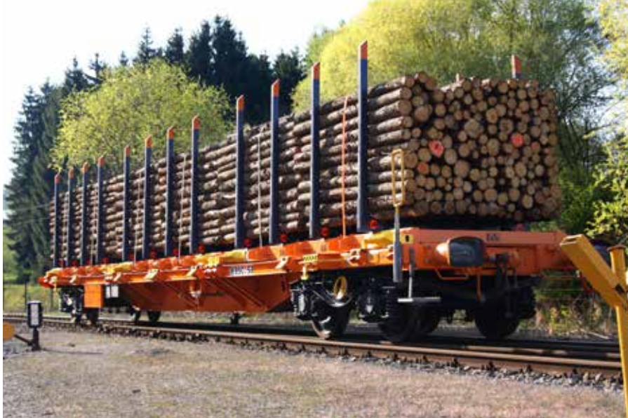
In the WASCOSA flex freight system®, the base unit without timber attachment can continue to be used at any time as a special freight wagon or as a fully-fledged 60t container wagon with further superstructure units.
