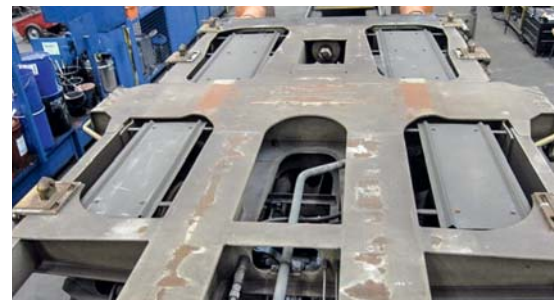
Figure 4 Spark-arrestor plate on freight wagon with K-block brake according to specifications still applicable today
