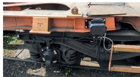
Figure 3 Diagnostic data memory and axle bearing generator with sensor system on a WASCOSA container car
