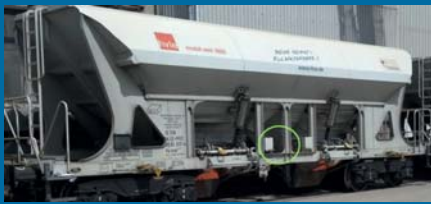
Figure 2 Equipment on freight wagons for automatic brake tests
