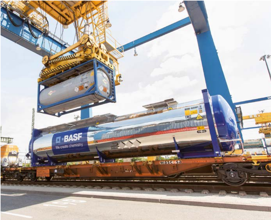
Fig. 1) 45-foot tank container optimised for rail transport (volume 63,000 litres, payload 66 tonnes). For size comparison on the left: a 20 foot tank container suspended from a gantry crane.
