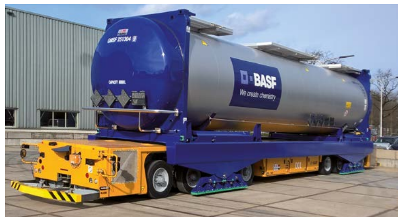
Fig. 2) First the AGV loads the blue subframe and sets the tank container on top, then proceeds the loading station.
