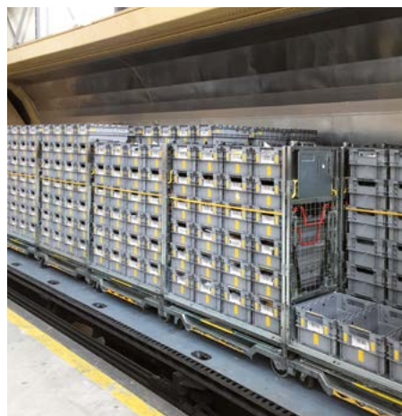
The interior of the wagon: the Habbiillnss loaded with pallets on wheels capable of holding up to 28 grey letter crates
