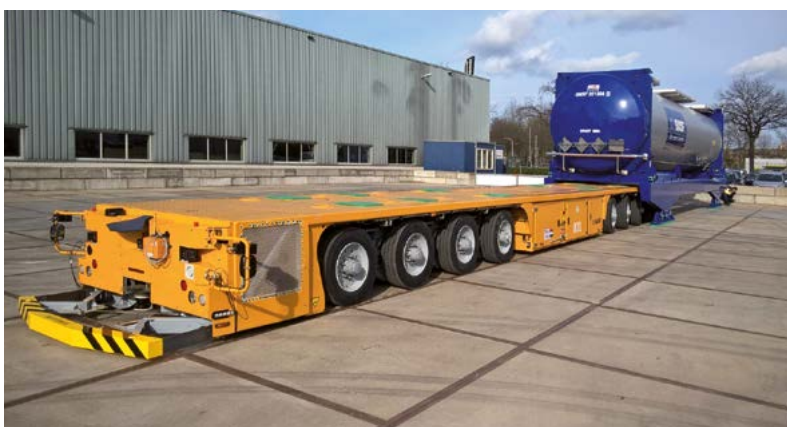
Next, the AGV lowers itself so that the blue subframe sits on the ground. The AGV then drives away from under the subframe ...
