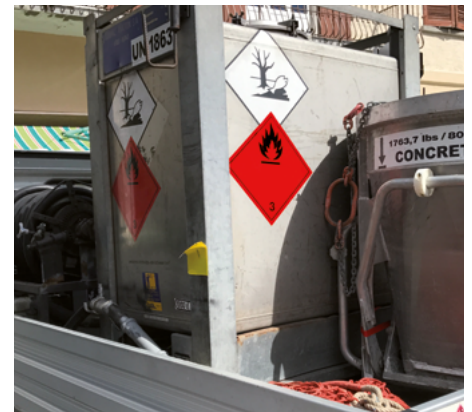
IB C with kerosene on a delivery van for mobile helicopter refueling. However, written with UN 1863 jet fuel.
