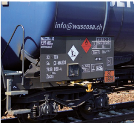
Delivery of fuel tanks with kerosene, but here not marked as UN 1223 but as UN 1863 marked by the refinery,
