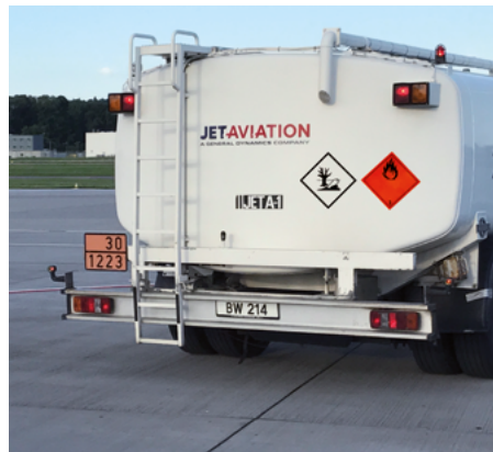
Labelling on tanker at Zurich airport is bang on: it contains kerosene (Jet A 1) for refuelling aircraft with jet or turboprop engines.
