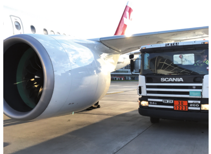
Miraculous transformation: UN 1863 in the storage facility suddenly turns into UN 1223 kerosene. This fuel is Jet A 1, which is classified as kerosene according to RID rules.
