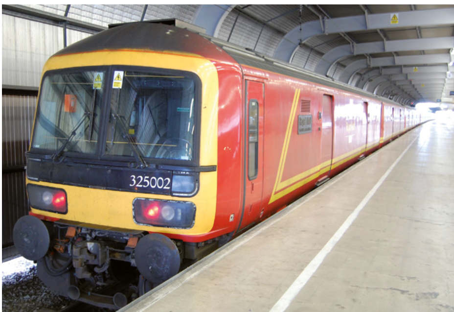
UK railway postal service at a terminal, DB Cargo UK class 325 EMU for 25 kV 50 Hz, Vmax 160 km/h, max. four wagons with automatic buck-eye coupling using multiple-unit train control, on the East and West Coast Mainline (photo: DB Cargo (UK) Limited)
