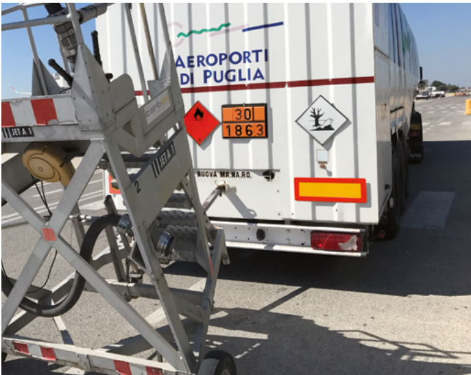
A common sight at airports: the tanker is labelled as UN 1863 rather than UN 1223 kerosene. This tanker was spotted at Brindisi airport.
