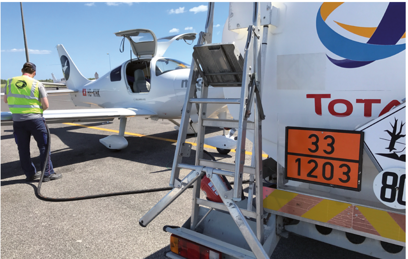
Light-sport aircraft being filled with aviation fuel UN 1203 (Avgas). Not to be confused with Jet A 1 – the consequences could be disastrous!
