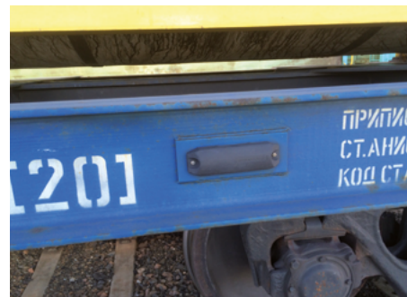
RFID for “wayside monitoring” has long been standard for Russian freight wagons (photo: the author, 2014)
