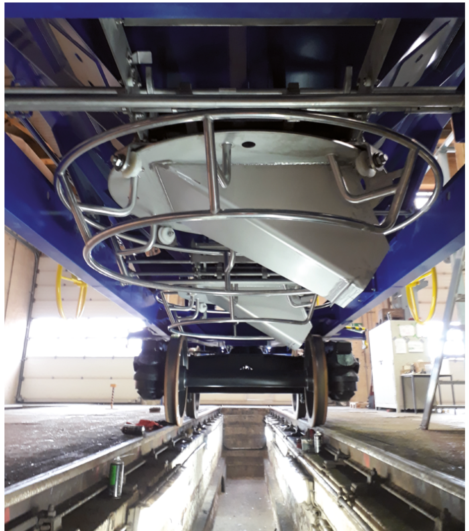
The Tanpps wagon offers fast unloading times and a high degree of flexibility, partly thanks to the unloading chutes that can swivel in three directions.
