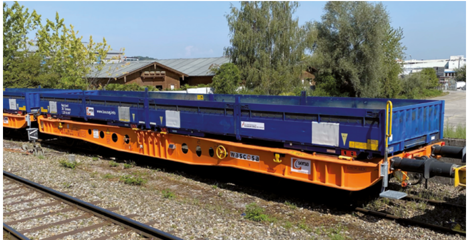
Wascosa's 48' Sgmmns multipurpose wagon with adapted swap platforms with tiltable sidewalls
