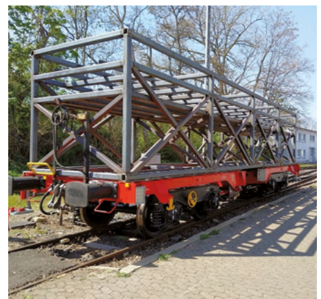
Preparation of tests with special container for simulating the worst-case load
