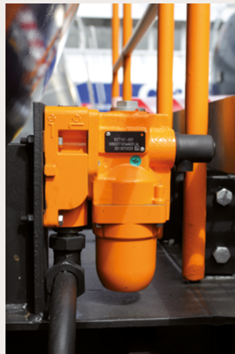
4. derailment detectors from Knorr-Bremse AG
