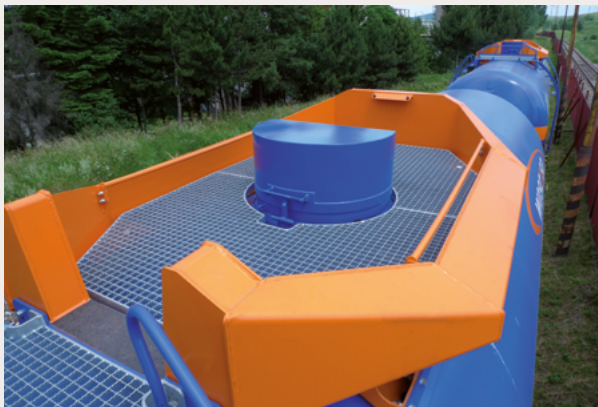
3. a rollover protection device (EST UE01) for the valves on top of the tank
