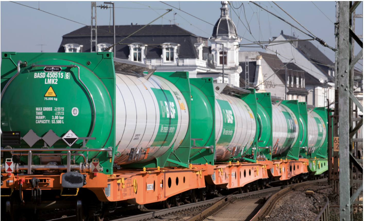
Example of innovation: Particularly quiet flat wagons designed, among other things, for transporting tank containers for chemical products
