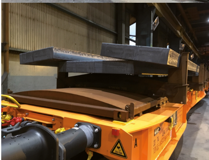
The Wascosa flex freight system® in use with superstructures for steel transport and rail infrastructure construction.
