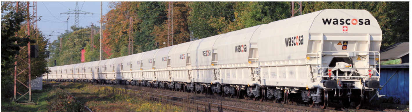
The brand new, white bogie bulk freight wagons Falns for thyssenkrupp Steel Europe.
