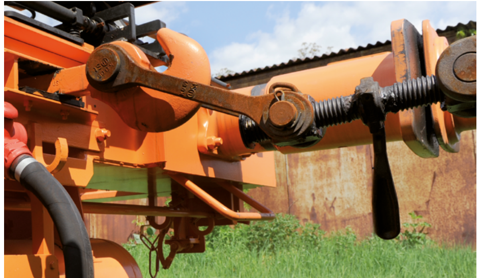
In rail freight transport, Europe is the last (entire) continent where screw couplings are still used.
