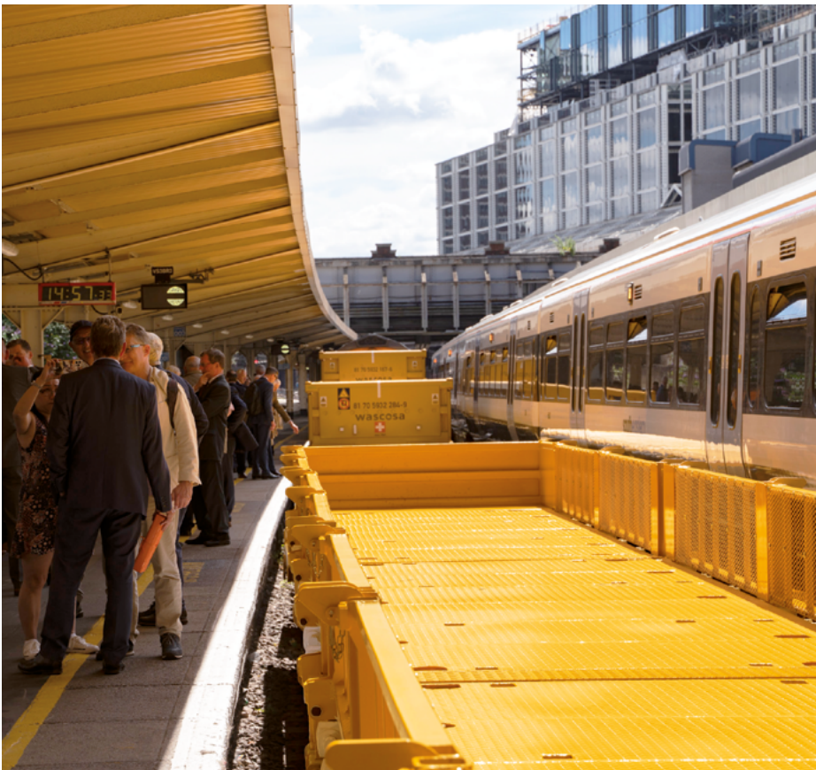
In the foreground: The Wascosa flex freight system® 60' container wagon with extended front ends and lateral flaps for transporting short rails and loose components.
