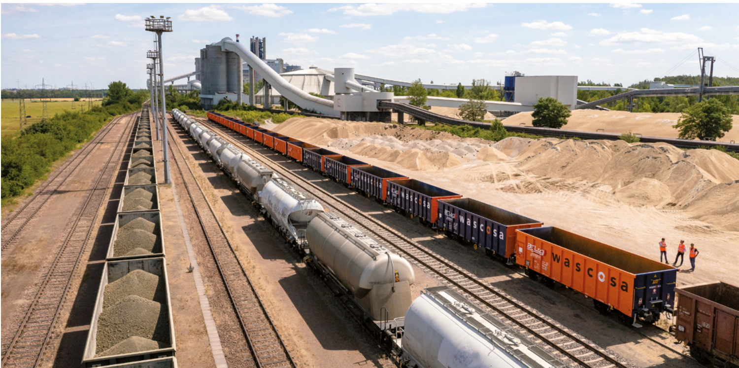
Wascosa's new Eamnos wagons (right) are used to transport sand to the south and bring back spoil.
