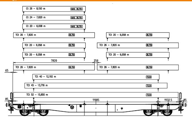
The Wascosa flex freight system® container flat wagon can be combined with the following superstructures
