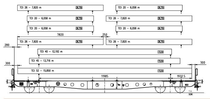
The Wascosa flex freight system® container flat wagon can be combined with the following superstructures
